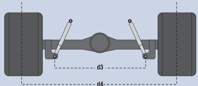
**Diagram 2 (Beam Axle Suspension)**
